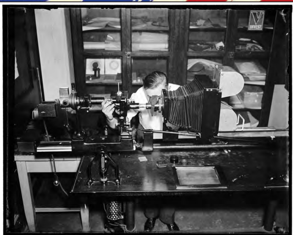
Bureau of Standards speeds up photomicrography with new apparatus. By means of this new apparatus just designed by the metallurgical divisions of the National Bureau of Standards, it is now possible to make 700 micrographs per working day of the structural effect of corrosion on cross sections of metallic specimens. This new machine uses roll film of 900 negatives at one loading, thus dispensing with the repeated loading and unloading of individual film holders by which method the Bureau was only formerly able to make 12 micrographs per working day. Willard H. Mutohler, one of the designers of the apparatus is shown photographing the corrosion on airplane materials, 8/18/37, Courtesy of Library of Congress, Photo by Harris & Ewing.
